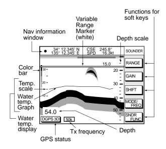
Figure 2-2 Indications on the normal sounder display
